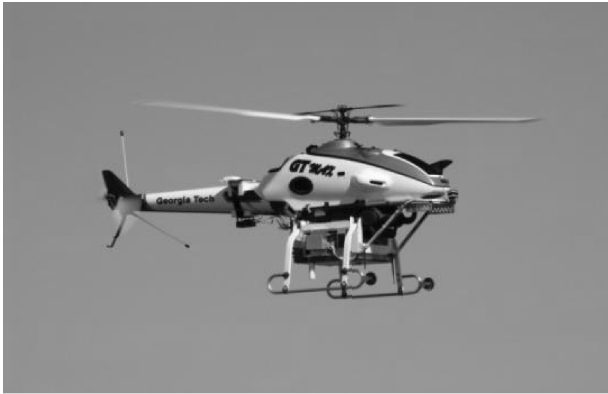
Fig. 9 Georgia Tech GTMax, in autonomous landing approach.
